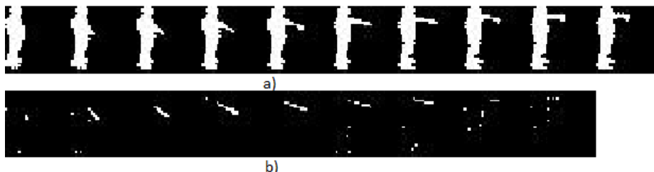
Fig. 5. a) The sequence of images depicting the check watch action; b) The sequence of images obtained by subtracting consecutive images of the check watch action.
