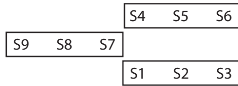
Figure 2: The figure shows what sensor number correspond to what sensor on LUCS haptic hand I. The view of the open robotic hand is to be considered as seen from above.
