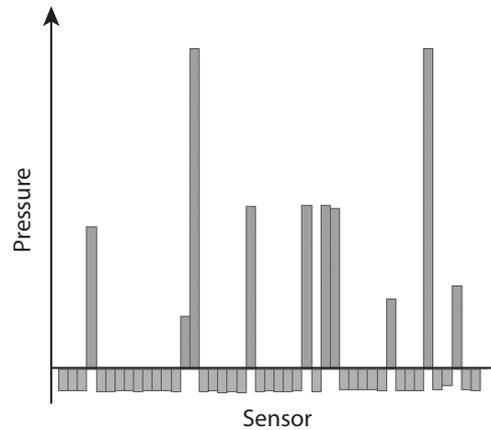
Figure 2: Signals from the Lucs Haptic Hand II during the grasping of an object.
