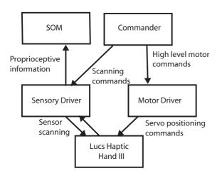
Figure 2: Schematic depiction of the single grasp model. The commander program executes the grasps by sending high-level motor commands to the motor driver, which translates and conveys the information to the servo controller board of the robot hand. When the robot hand has become fully closed the commander program request a scanning of the registers of the 11 proprioceptive sensors of the robot hand. The sensory information is conveyed as a vector to the self-organizing map.
